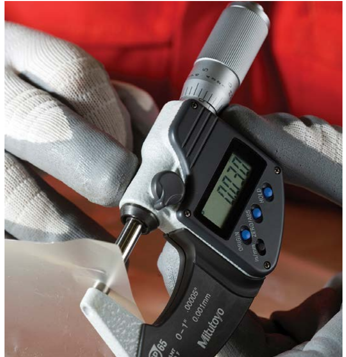
Measuring the thickness of extruded APTIV Film.
