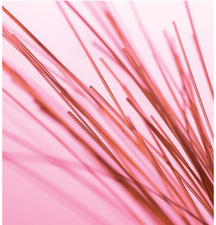
Extruded VICTREX PEEK fibres.
